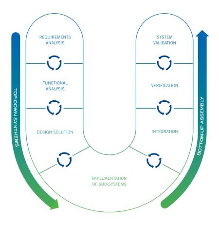
Figure 1: Vee model of system engineering.
